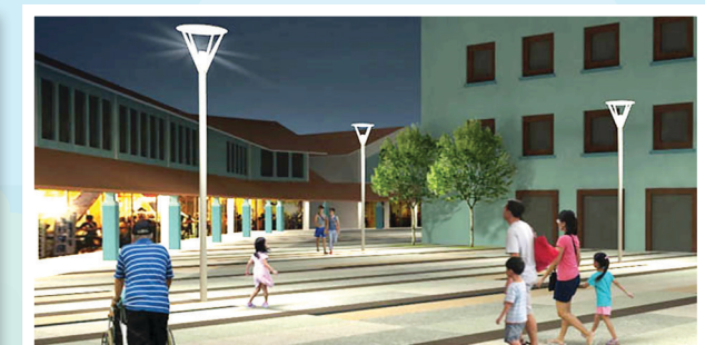
New lamp posts with reflectors to provide softer light
